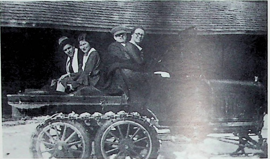
"The Snowbird", modified Model T Ford, with track drive for traction on ice and snow, a forerunner of the snowmobile, March 21, 1931. Occupants are (left to right) Donald Smith (Janey's nephew), Stella, Willie and Janey Shearer. Willie used the Snowbird for deliveries from his Lakehurst store in winter and rarely, if ever, was prevented from doing so. The vehicle was a source of community reassurance during winter storms. N.B. (background) Old Lakehurst store.
