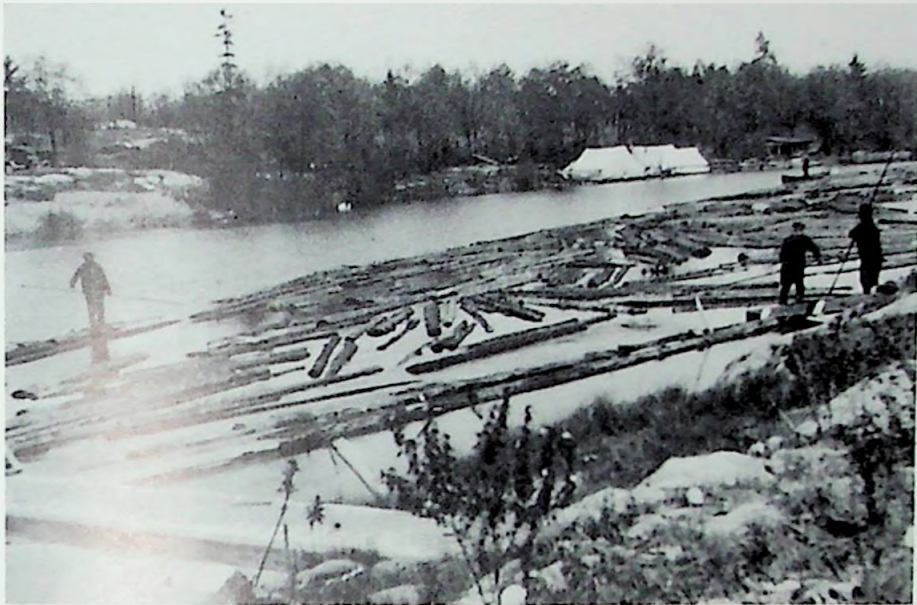
Marshalling logs by Mississauga (Gull) Lake dam ( left ) during log-drive of 1923. N.B. River-drive with pike-poles for pushing and controlling floating logs; rafts in background with tents for mobile cookhouse and sleeping quarters; small trees probably second growth after logging and fire; bare rocky land.
