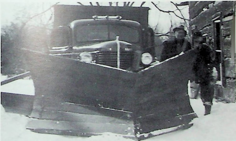
The first truck-powered snowplough in Harvey belonging to Willy Shearer of Lakehurst. The plough was of shaped lumber bolted to a metal frame mounted on the REO truck. One of the two men is Wilson Blewett. (Courtesy Clara Telford).
