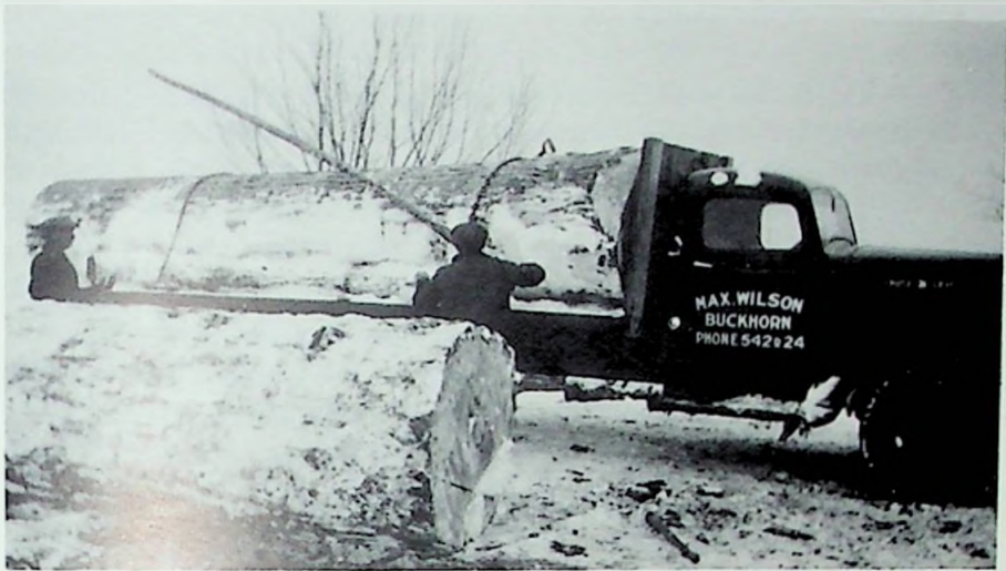
Logging with trucks, 1939. Large elm log cut by Ralph Garbutt, loaded by Walter Harrison, for Wallace Sugarer's mill. N.B. Binder pole to tighten chain around log.
